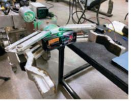
The team designed and engineered a revolutionary device which enables operators to sense the depth between an EOD robot's gripper and an object of interest, enhancing the driver's spatial awareness and accelerating counter-IED operations overall.
